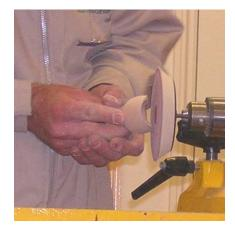
In case the Jacob's chuck has a mind to come out, you can retain it in place by having the toolrest in it's path , blocking it's way if it comes loose.
