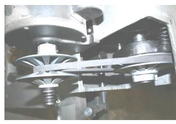
I decided to pull the converging cone arrangement off their shafts, to make fitting the new belt easier. I found that cones, which
