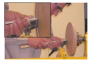
Now to the cutting in of the cove on the front face. This is of course optional, but adds a bit of decoration in what would otherwise be a glorified round plank, and will catch meat juices if you're making a carving board. I never much fancy using wood as a medium for carving meat on, but I suppose I am weird. Anyway, the cove...
