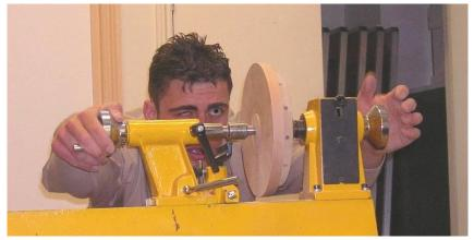
If you've marked out the centre of the workpiece in advance, it should run reasonably true once it is mounted.
